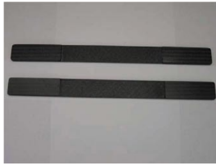
Figure 7. Specimens' avg. thickness - left: autoclave (2.23 mm); right: microwave (2.77 mm).
