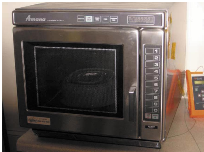
Figure 3. 2.45-GHz commercial microwave oven and temperature data recorder.
