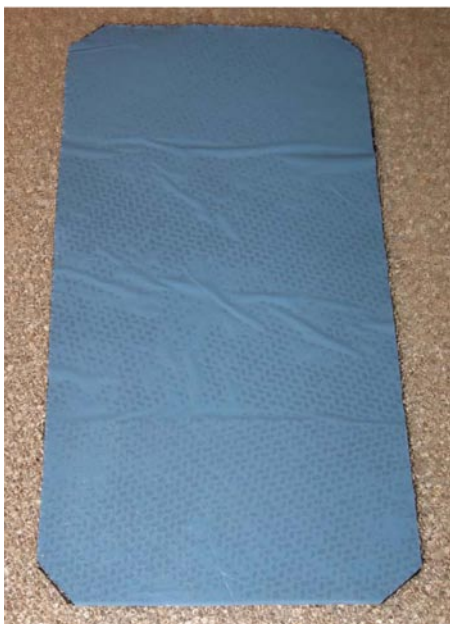
Figure 4. – Trimmed slab with minimum 2 mm (0.079 in) thickness.
