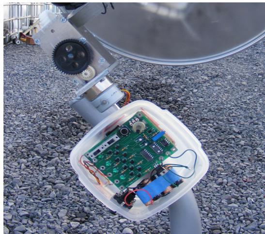
FIGURE 3. STIRLING ENGINE TRACKING DEVICE.
