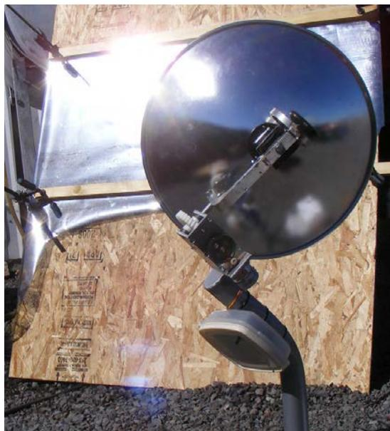
**FIGURE 1. TYPICAL FIELD TEST ARRANGEMENT, SHOWING THE SAMPLE REFLECTING FILM UNDER TEST, THE STIRLING ENGINE WITH ITS PARABOLIC CONCENTRATING DISH, AND THE TRACKING DRIVE.**
