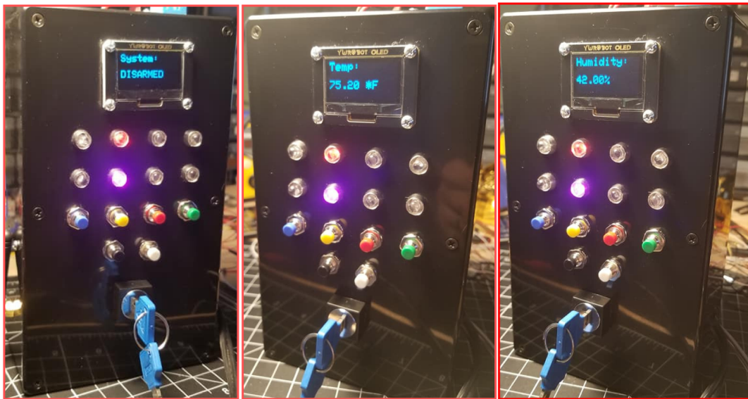
Figure 12. The system status (Disarmed) and laboratory environmental parameters on the OLED. OLED, organic light-emitting diode.
