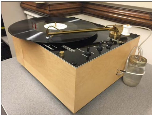
Machine cleaning a transcription disc. Photo by Cristina Kühn.
