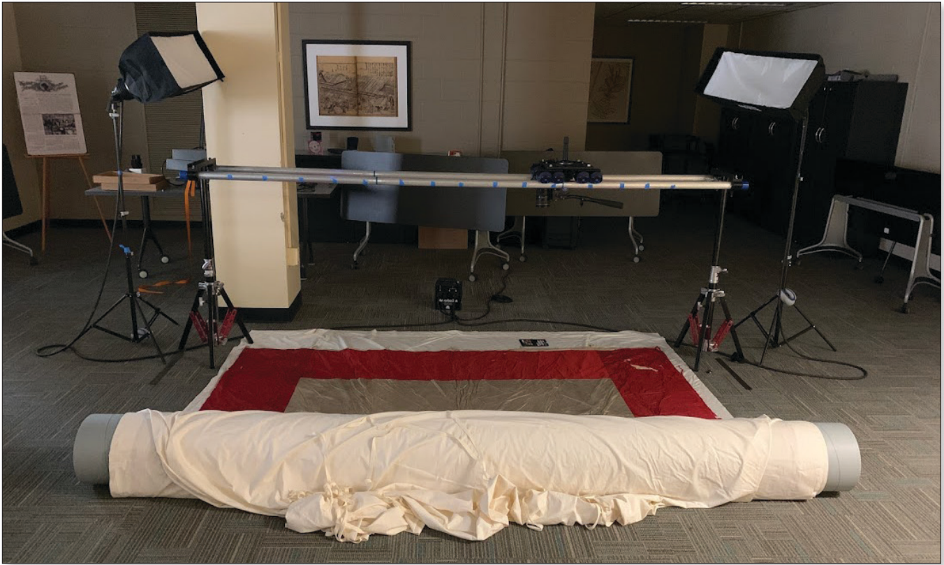
Evolved digitization setup using a camera dolly and dolly track for documenting the fragile WWI-era banner. Photo courtesy of Crystal Heis, UK Libraries.
