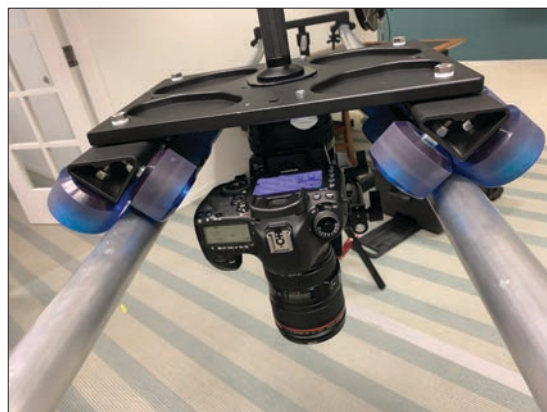
Camera dolly with modified camera mount. Photo courtesy of Crystal Heis, UK Libraries.
