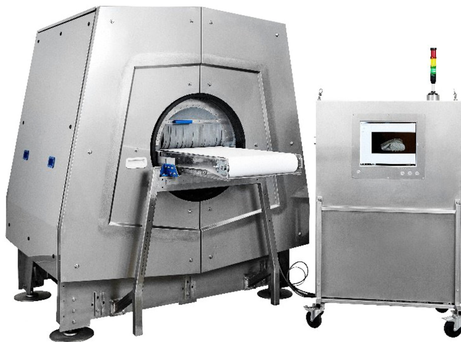
Figure 5. A prototype for online CT scanning. The prototype works at a line speed that matches 600 middles per hour and produces complete 3D images of each slice with enough resolution to distinguish the different tissues.
