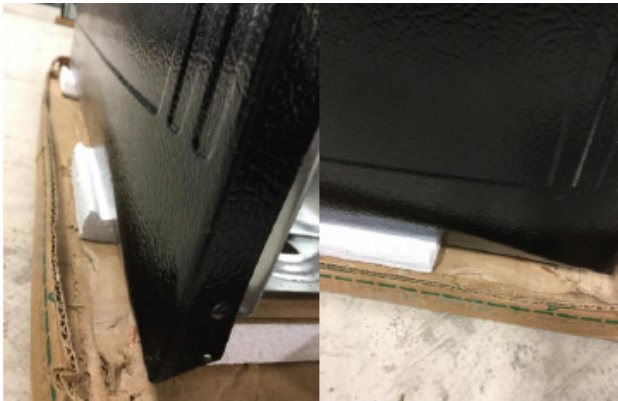
FIGURE 2: DROP DAMAGE TO SIDE PANEL
