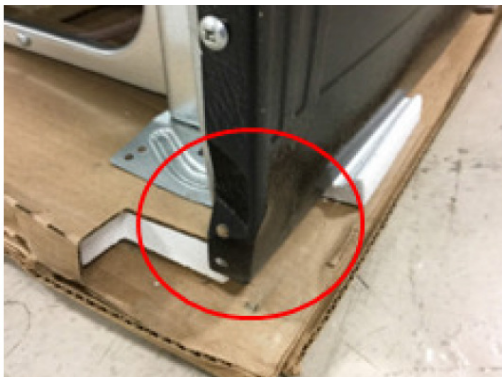
FIGURE 3: SIDE INCLINED IMPACT DAMAGE
