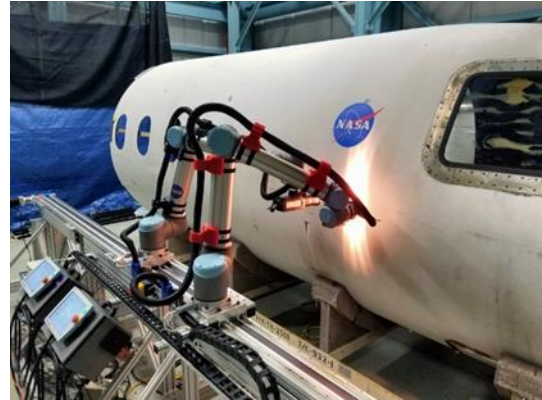
FIGURE 1: DUAL COLLABORATIVE ROBOTS INSPECTING A COMPOSITE AIRCRAFT FUSELAGE USING LINE SCAN THERMOGRAPHY.
