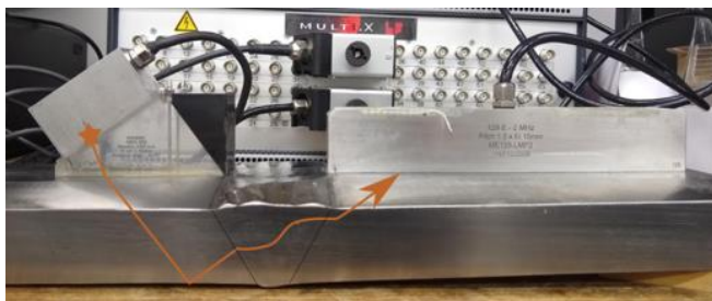
FIGURE 1: Experimental setup for ultrasonic weld characterisation.
