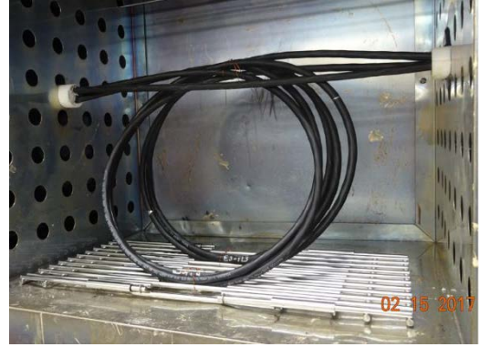
FIGURE 2: CABLE PLACED IN AIR-CIRCULATING OVEN FOR AGING
