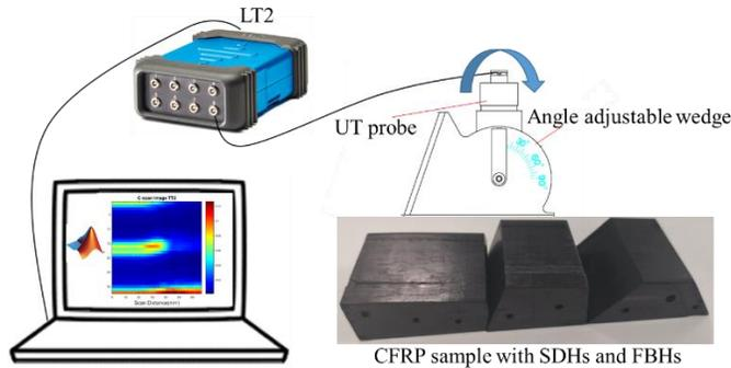
**FIGURE 3:** EXPERIMENTAL SET-UP FOR DEFECT DETECTION IN COMPOSITES
