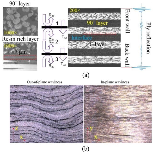
**FIGURE 1: (A) WAVE PROPAGATION IN COMPOSITES AND (B) WAVINESS AND DELAMINATION IN COMPOSITE OBSERVED FROM MICROSCOPE**
