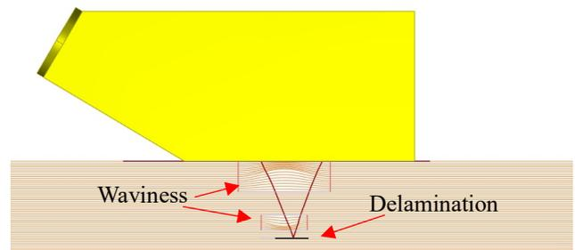
**FIGURE 2: NUMERICAL MODEL FOR WAVE INTERACTION WITH DELAMINATION WITHIN WAVY COMPOSITE**
