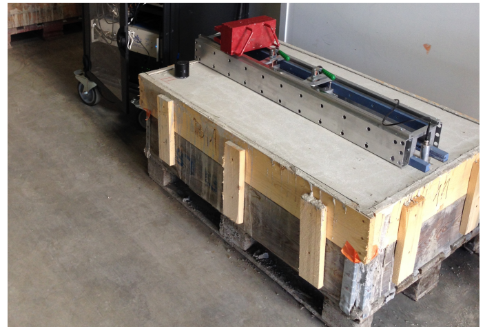
FIGURE 4. ULTRASONIC MEASUREMENTS ON CONCRETE.
