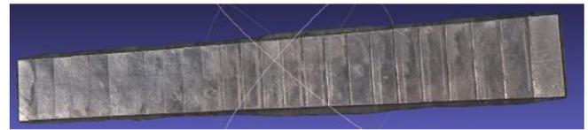
**FIGURE 2: MESH OF ALUMINUM STAIR.**
