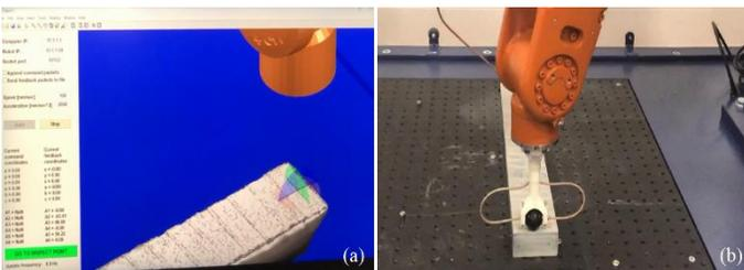
**FIGURE 5:** VISION GUIDED ROBOTIC COMPONENT NDT INSPECTION: AN OPERATOR SELECTING A POINT ON THE SURFACE OF THE 3D MODEL INSIDE THE GUI (A) AND ULTRASONIC WHEEL PROBE APPROACHES ALONG THE NORMAL OF THE POINT FOR DATA MEASUREMENT (B).
