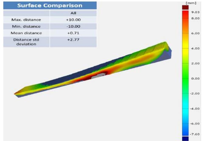
**FIGURE 3: SURFACE ANALYSIS OF THE ALUMINUM STAIRS MESH ON ACTUAL CAD.**
