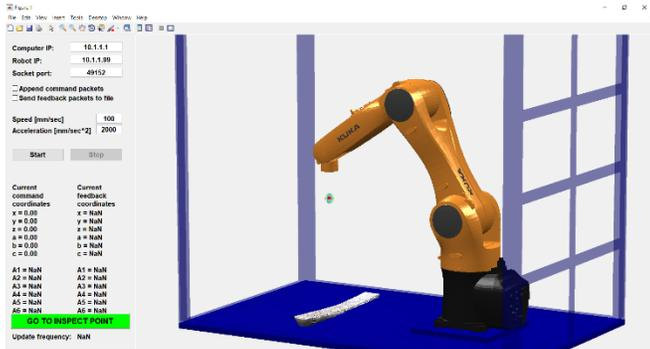
**FIGURE 1: GRAPHICAL USER INTERFACE TO IMPORT THE RECONSTRUCTED PART GEOMETRY AND EXECUTE VISION-DRIVEN NDT INSPECTION.**
