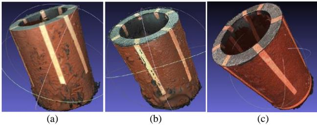
**FIGURE 4:** RESULTANT MESHES OF THE PIPE SEGMENT FOR THE THREE IMAGE ACQUISITION APPROACHES: POLAR RASTER (A), HEMISPHERICAL SPIRAL (B) AND PARABOLOID SPIRAL (C).
