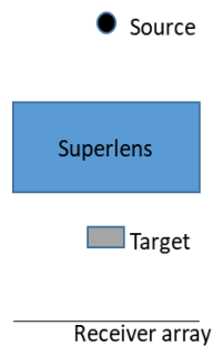
FIGURE 2: PROPOSED MICROWAVE NDE SYSTEM USING A METAMATERIAL LENS
