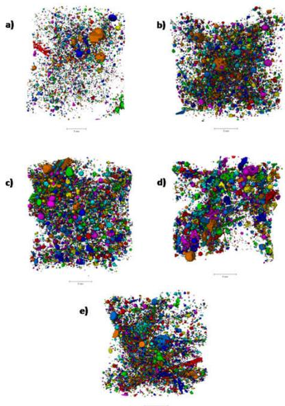
**FIGURE 3: 3D GRAPHICS MODELS FOR PORES: a) Y1, b) X1, c) X2, d) X3 and e) X4**
