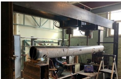
FIGURE 3: HDPE PIPE UNDER FOUR-POINT BENDING
