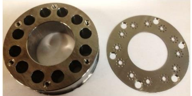
Figure 1. Photograph of the annular phantom body (left) and cover.
