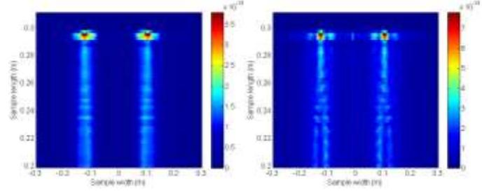
**FIGURE 2:** TR ENERGY FOR VARYING METAL LENGTHS, (LEFT) LENGTH: 5 CM, (RIGHT) LENGTH: 40 CM
