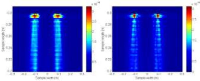
**FIGURE 3:** TR ENERGY FOR VARYING METAL SEPARATION, (LEFT) GAP: 6 CM, (RIGHT) GAP: 8 CM
