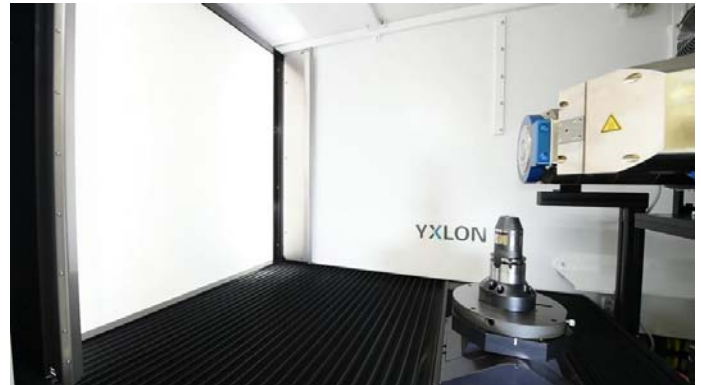
FIGURE 1: Inside CT system, left: white screen, middle: object stage, right: x-ray tube
