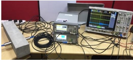
Figure 1: ULTRASONIC TESTING ON CEMENT COMPOSITE SPECIMEN
