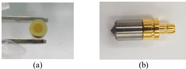
FIGURE 3: Image of fabrication process of ZnO piezoelectric transducer (a) ZnO piezoelectric element and (b) Sensor casing
