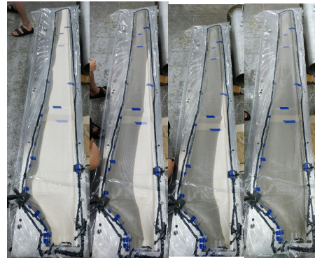
Fig. 2 Fabrication of wind blade skin
