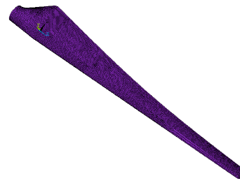
Fig. 3 FEM model of blade
