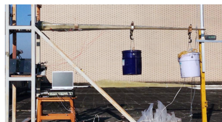
Fig. 4 Static load testing of blade
