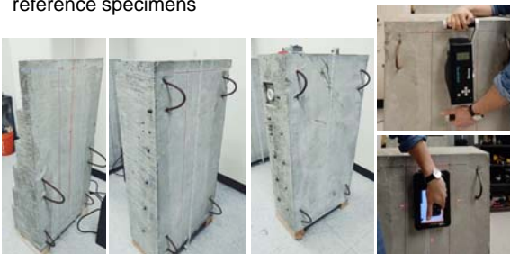
Reference specimens set up in the laboratory for taking measurements: Specimens 1 to 3 (from left to right). Top right: ultrasonic array instrument, bottom right: radar instrument.
