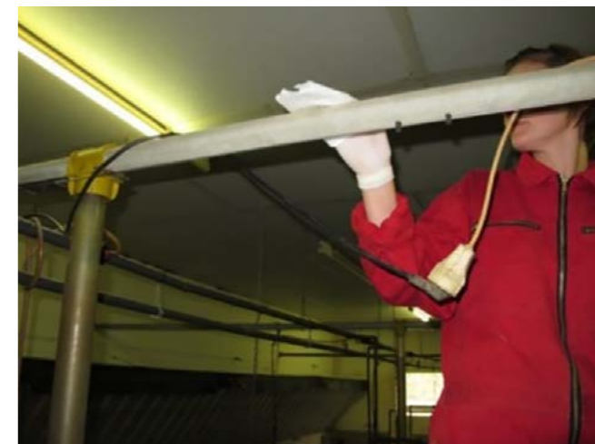
Photo 2: Collecting a dust sample for bacteriological investigation
