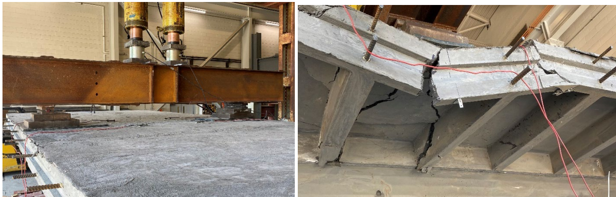
Figure 7: Ribbed slab test setup and failure mode
