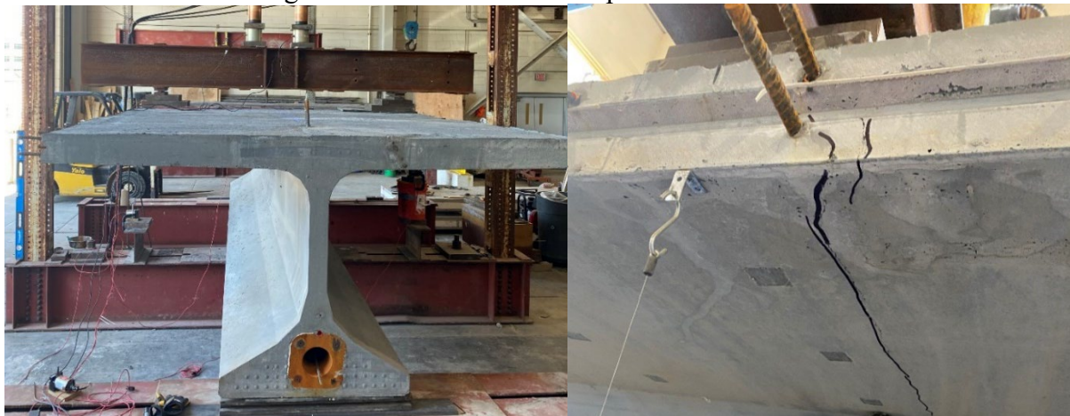
Figure 8: Solid slab test setup and failure mode
