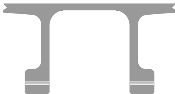
Figure 3. Cross-section of a Pi or double T beam. Taken from: Advanced Concrete Modular Systems Catalog, Argos.
