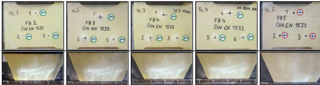
Figure 2: The front (top) and back (bottom) faces of sandwich structures tested to EN 1522:1998.
