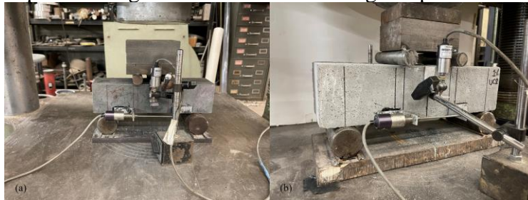
Figure 1. Full test setup for (a) 3-in. by 3-in. by 12-in. and (b) 4-in. by 4-in. by 15-in. prisms
