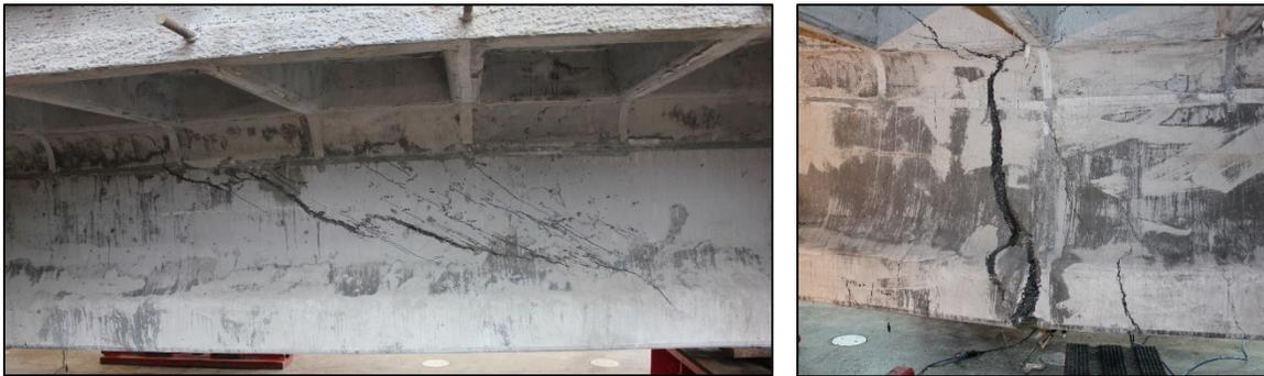
Figure 8: Shear Tests without Stirrups (left) and with Stirrups (right)
