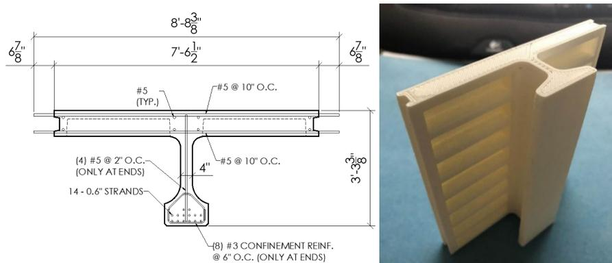
**Figure 1: Full-Scale UHPC DIB Tested, cross-section (left), 3D printed model shows waffle slab (right)**
