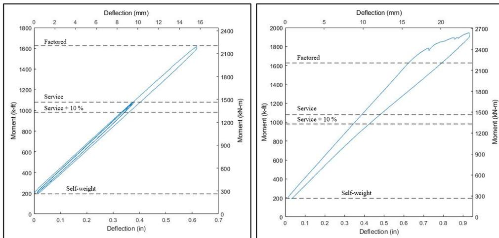
Figure 7: Moment vs. Deflection Plots for to Factored Load (left) and the Cycle beyond Factored (right)
