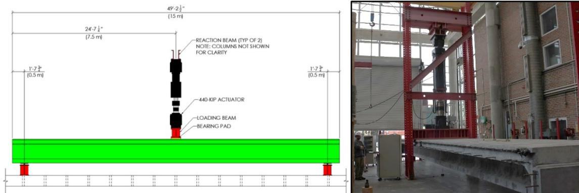
Figure 6: UHPC DIB Flexure Test Schematic (left) and Setup in the Laboratory (right)
