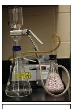
Figure 3. Vacuum filtration test setup.
