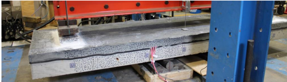
Figure 2. Example of conventional concrete slab with UHPC overlay in test frame
