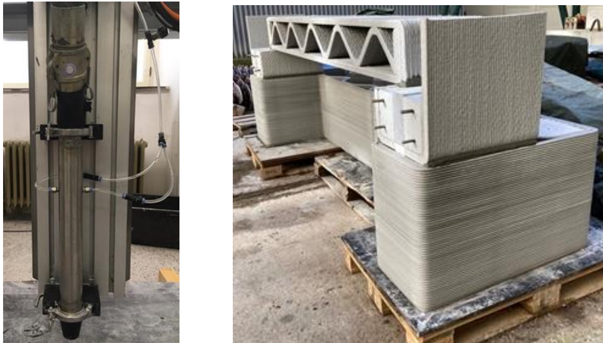
Fig. 1: The print head of the TestBed device in KI on the left, the printed object in the 3D STAR project on the right
