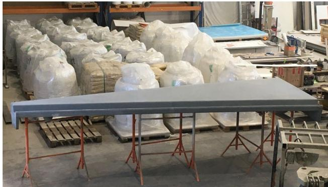
Figure 4: Tile just demolded – geometric control
