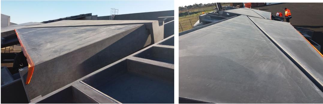
**Figure 9: Tests at Innobéton factory: tolerance in case of settled support**
