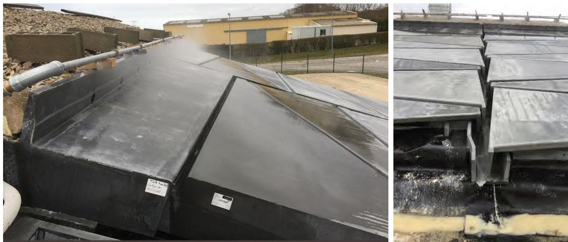
Figure 13: Full-scale test of water runoff and channeling
