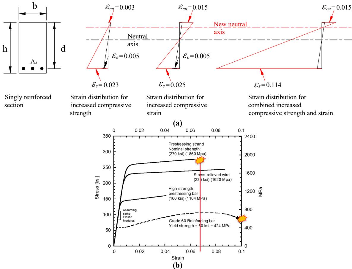
Figure 5: (a) tensile strain demands in the longitudinal steel reinforcement caused by the maximum compressive strain of UHPC, (b) strain capacities of typical prestressing strands and rebars
