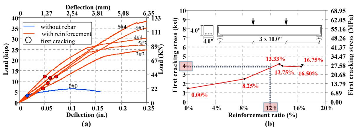
Figure 6: (a) test results, (b) first cracking stress versus reinforcement ratio ( $\rho_{TA}$  = rebar area divided by the “tributary area of concrete” =  $2 \times$  cover thickness  $\times$  width of beam)
