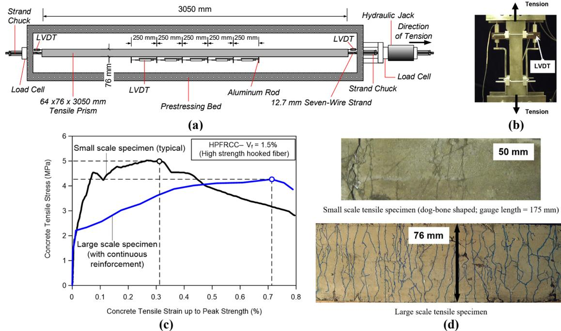
Figure 2: (a) larger-sized tensile specimen (with continuous steel reinforcement), (b) smaller-sized tensile specimen, (c) comparison of stress-strain responses between smaller- (no continuous steel reinforcement) and larger-sized specimen, (d) crack distributions in smaller- and larger-sized tensile specimens (Chao et al., 2007)
