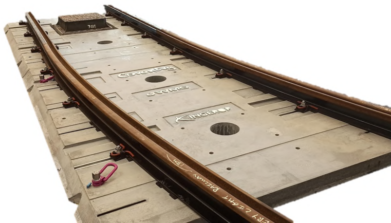
Figure 6: The integrated cast-in channels within the UHPC slab allow for rails to have any curved alignment without the need for a bespoke slab to be cast for each uniquely shaped section of the route.
