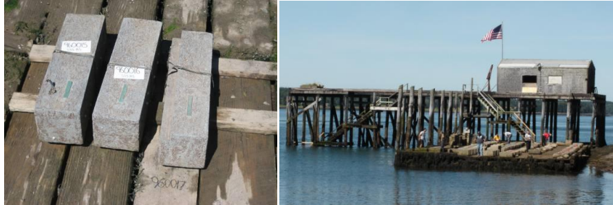
Figure 1: UHPC Prisms (left) at the US Army Corps of Engineers Treat Island Marine exposure station (right), Maine, U.S.A.
