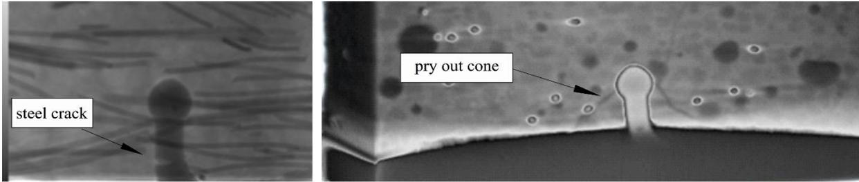
Figure 6. Results of CT scans in UHPC (left) and HSC (right).
