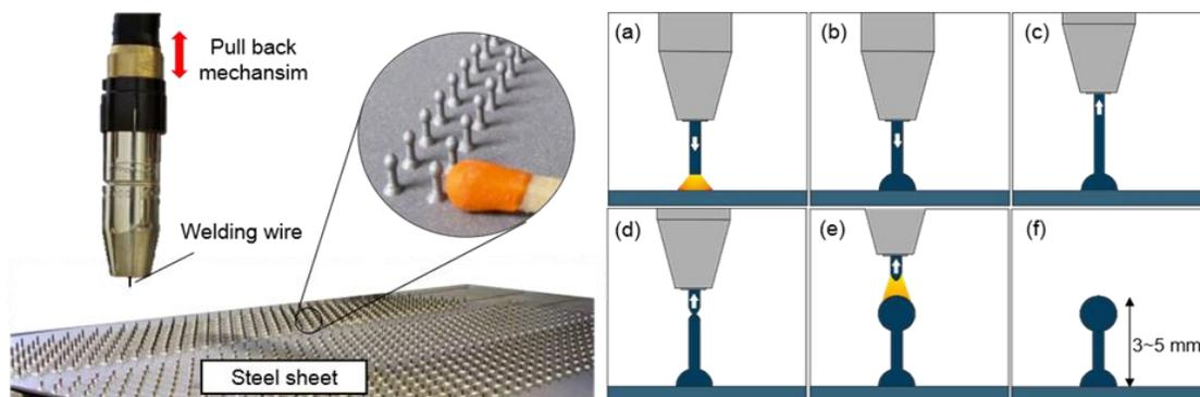
**Figure 2. Schematic diagram of the CMT welding with illustration of the dropping process (Bruckner, 2005).**
