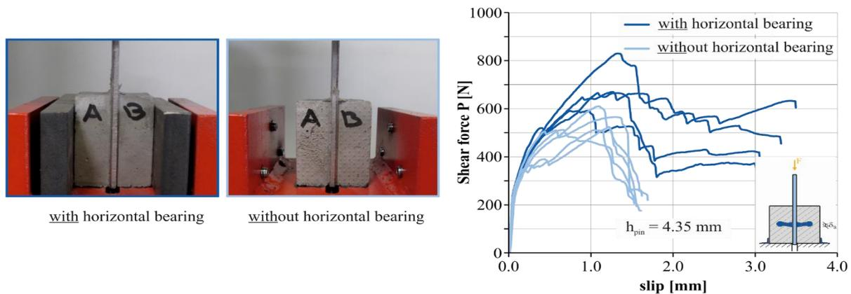
**Figure 4. Shear tests: experimental setups (left), force-slip relationship (right).**
