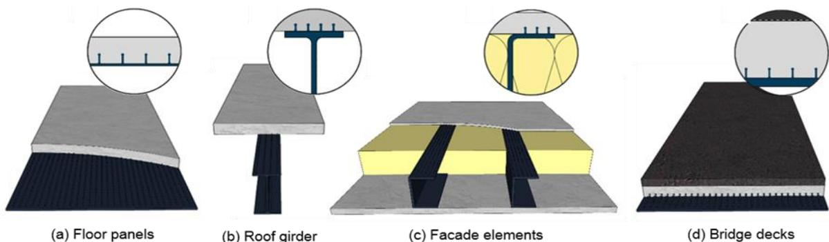
Figure 1. Applications for small-scale shear connectors.
