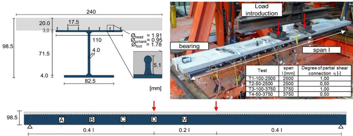
Figure 7. Dimensions of the cross section and test setup of the composite beam tests T1 – T4.
