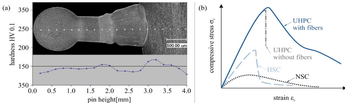
**Figure 3. Hardness testing on a pin (a), stress-strain relationship of various normal and high strength concretes according to (Leutbecher, 2008) (b).**
