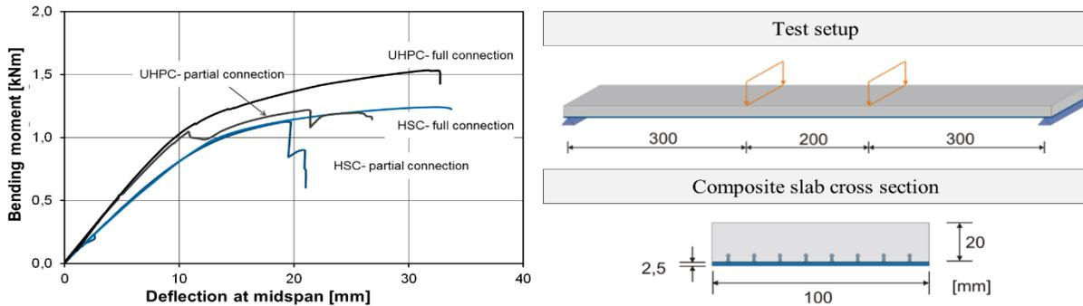
Figure 5. Experimental results of composite slabs (left), static system and cross section (right).
