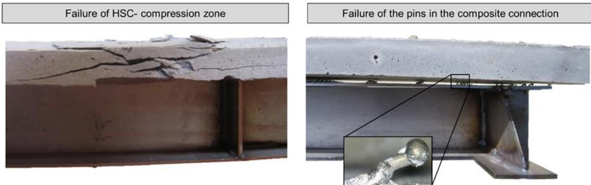
**Figure 9. Failure of HSC- compression zone (left); Failure of the pins in the composite connection (right).**
