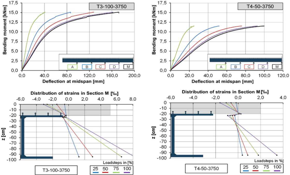
**Figure 8. Bending moment-deflection curves at midspan (top) and strain distribution (bottom) of the beams T3 (left) and T4 (right).**
