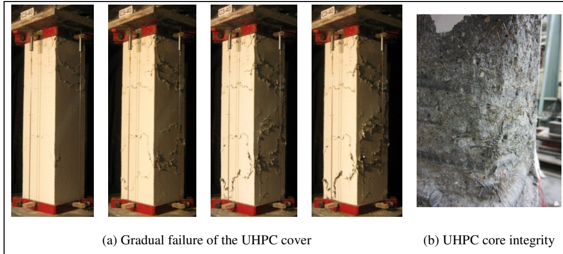
Figure 5. Controlled failure of cover and core in UHPC columns (Column C3-40)
