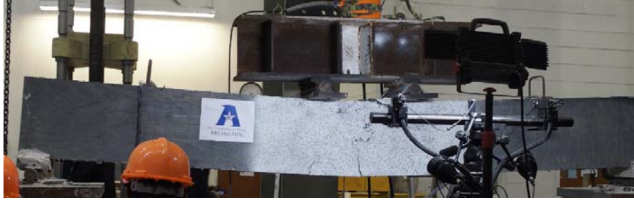
Figure 9. Large deflection in UHP-FRC beam
