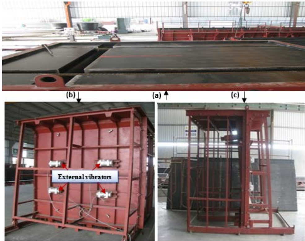
Figure 6. (a) Top view, (b) Front view, and (c) Side view of steel mold
