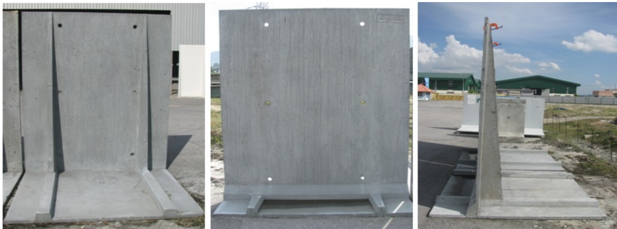
Figure 7. Back view (left), front view (middle) and side view (right) of precast UHPC retaining wall specimen
