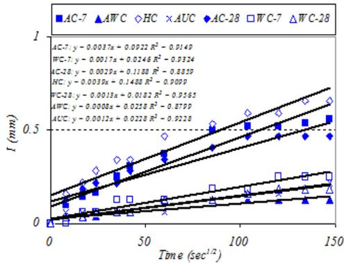
Figure 4. Initial water sorption of UHPC mixes
