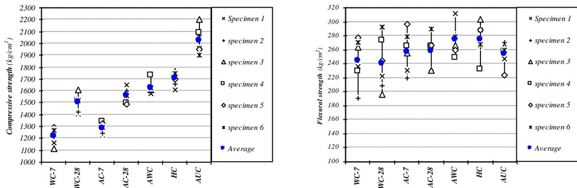
Figure 2. Compressive and flexural strength for UHPC mixes in different curing regimes
