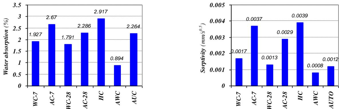
Figure 3. Water absorption and sorptivity of UHPC mixes
