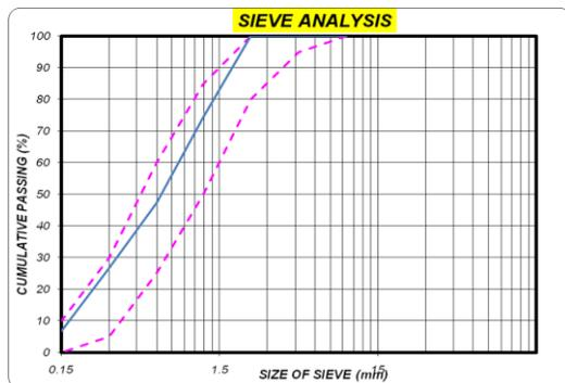
Figure 1. Grading curve of natural river sand
