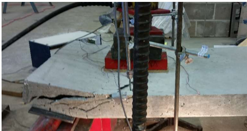
(a) Diagonal Tension Crack in a CC Control “Shear Panel” Test
