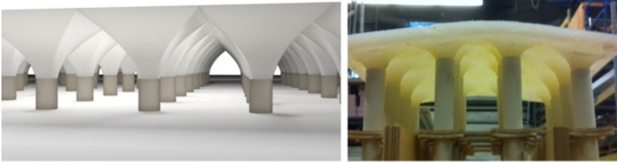
Figure 6: Variable stiffness of membrane created by sectional depth
