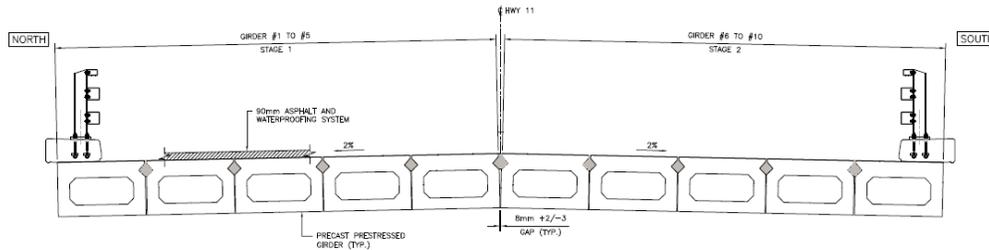
**Figure 2.** Typical MTO Adjacent Box Girder Bridge Deck Cross Section
