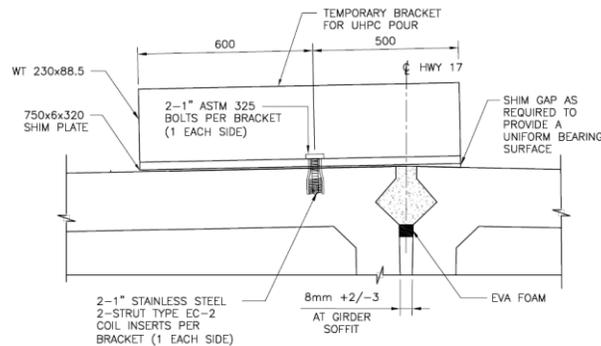
**Figure 9.** Temporary Centreline Joint Brace Detail
