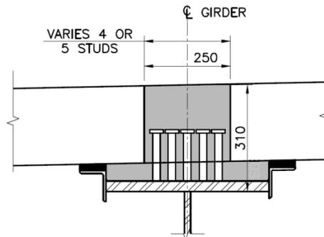
Figure 6. Typical Composite Connection Detail
