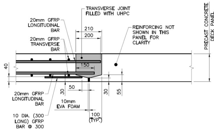
Figure 5. Typical Precast Deck Panel Joint Detail
