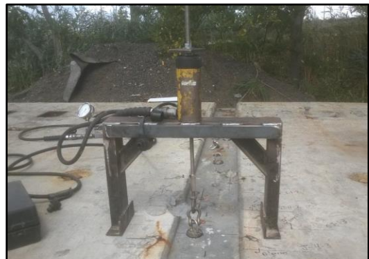
Figure 10. Pull-Off Test Setup
