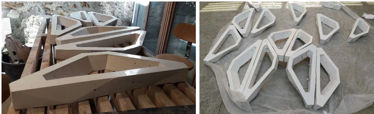
Figure5. First cast elements
