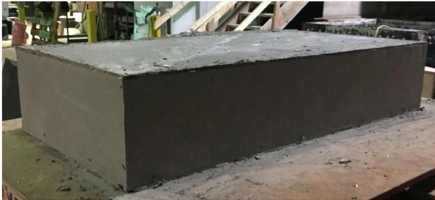
Figure 7 – UHPC Base Before Removing from Centre Forms
