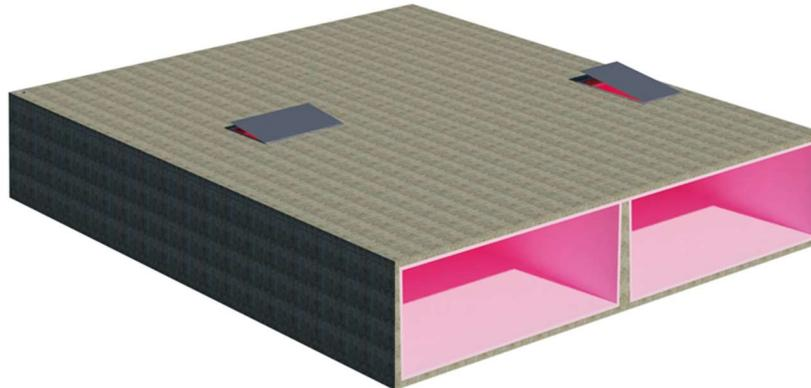
Figure 6 – Section of Concrete Floating Base
