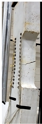
Figure 4. Out of plane bending observed during a 4 in. x 4 in. specimen test
