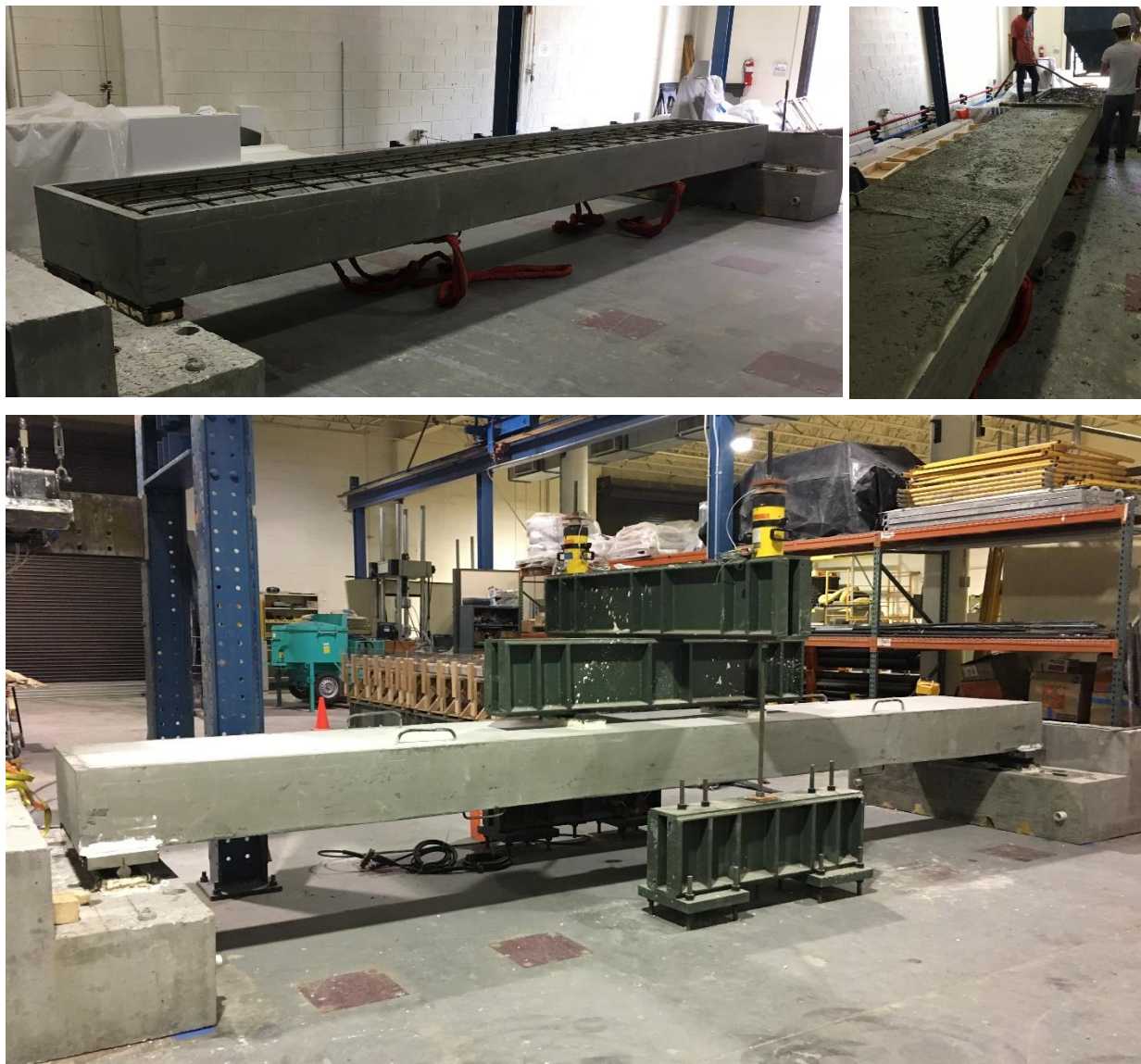
Figure - Construction and test set-up of specimen at Florida International University.
