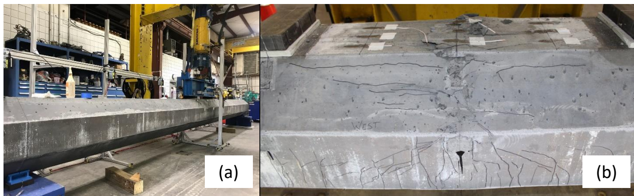
Figure 5. Flexural testing set up at FDOT Structures Research Center. Crack pattern at mid-span below point of loading.
